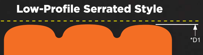
Fig. 5 - Low-Profile Serrated Style (*D1 = Tool Cutting Diameter)
